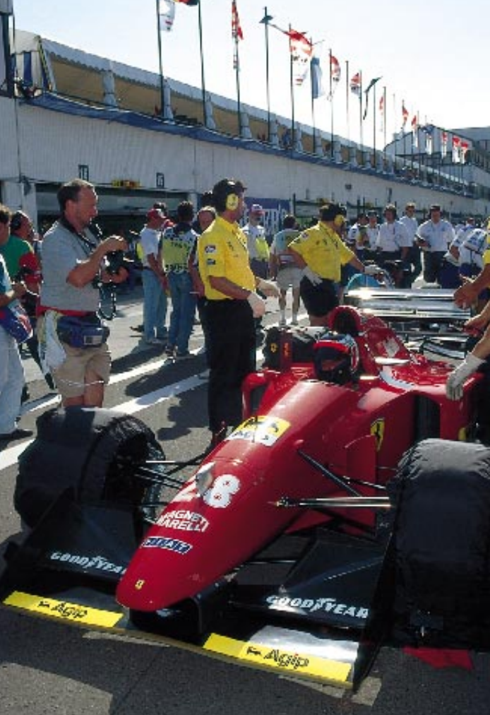
Gerhard Berger in the pits during the qualifying stages of the Hungarian Grand Prix. Electric tyre blankets cover the tyres to bring them up to racing temperature.
