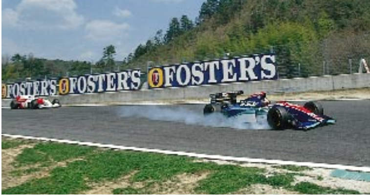
Rubens Barrichello applies his brakes late and hard as he drives into a sharp corner in the Pacific Grand Prix at TI Aida. In this case the wheel locks briefly and the tyre rapidly wears out on the locked area to create a 'flat spot'.
